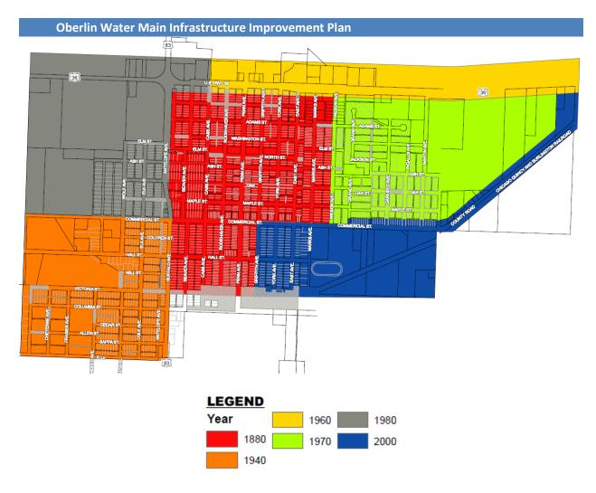
Above is a map of all of Oberlin's water mains sectioned out in the timeframes they were installed. Oberlin has been on an aggressive water improvement plan since the well project 9 years ago. Since then, the council has been dedicated to continuing with the much need upgrades and repairs to the City's water main system.
